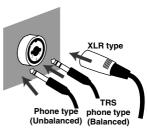
Both balanced and unbalanced connections are possible.
